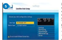
If Switch Type displays "SWM" or if given the option of selecting a Switch Type, select **Multiswitch**. Then, set the Dish Type for **Round**, **18"**, **Single LNB**, or **1 SATELLITE**,
